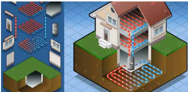
Heat can be transferred from below ground into underfloor heating.
